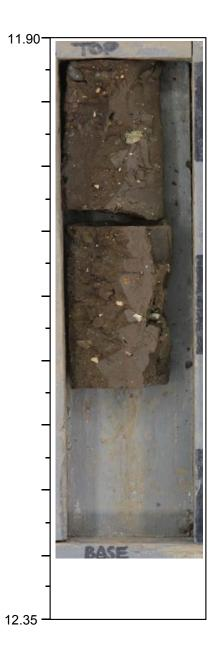
12.23 - 12.35m: Sample unavailable due to lab testing.
